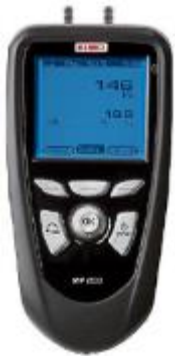
Mobile recorder thermo-Anemo-Manometer with backlit graphic display. Functions: Pressure, Temperature, Speed and Flow by Pitot tube
