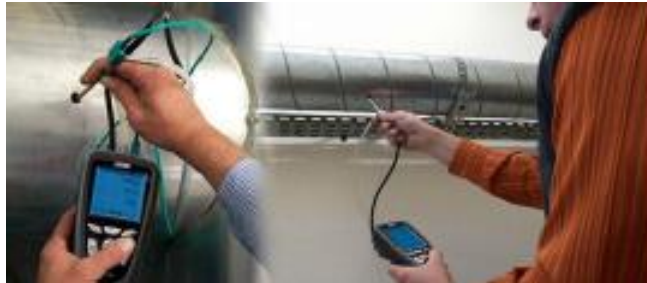
Mobile recorder thermo-Anemo-Manometer with backlit graphic display. Functions: Pressure, Temperature, Speed and Flow by Pitot tube
